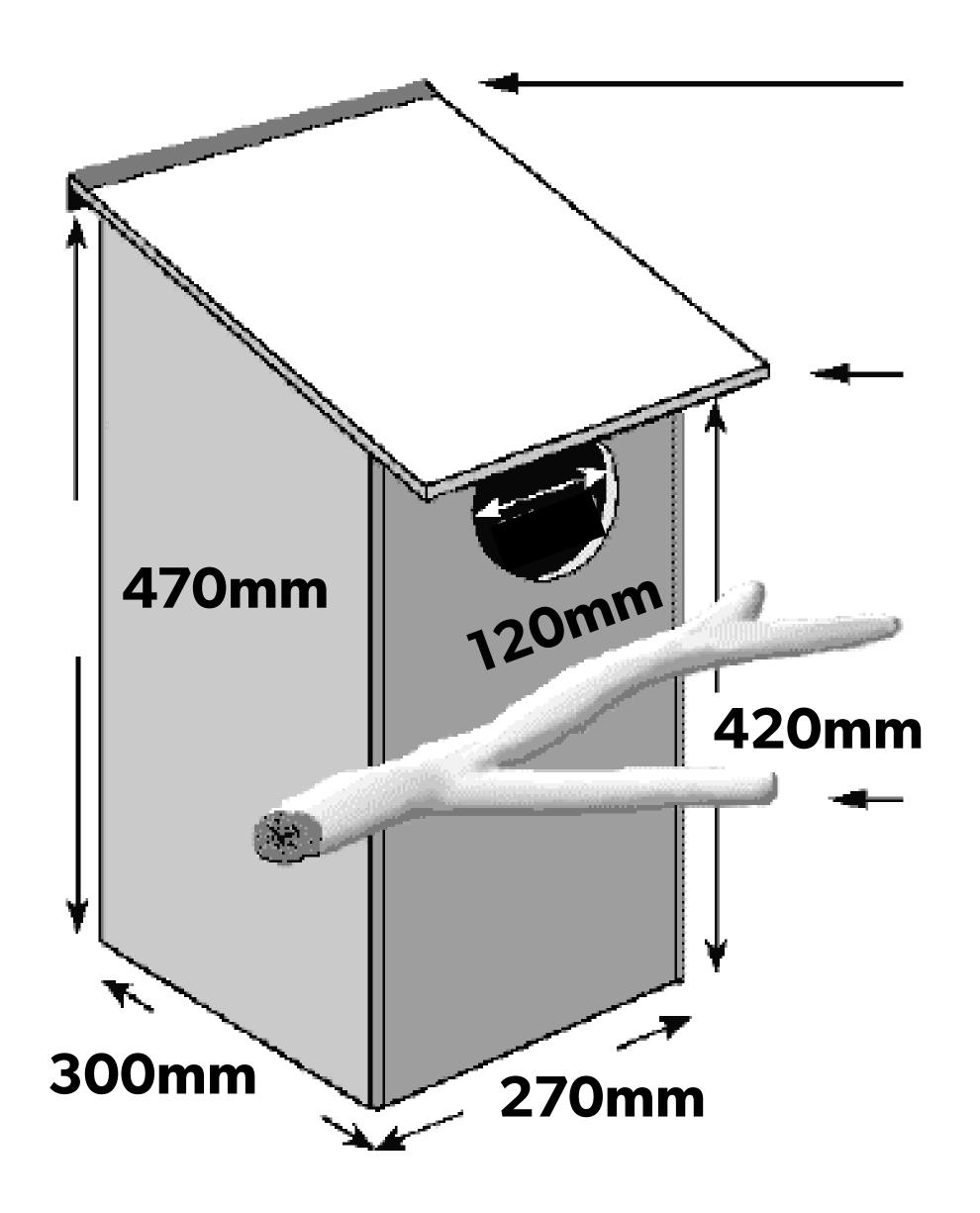
The top edge of the roof should be weather sealed with a folded strip of sheet metal, aluminium angle or a rubber flap.
