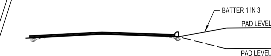
TYPICAL BUILDING ENVELOPE LOT / PAD LEVEL DETAIL 1 SCALE: INDICATIVE
