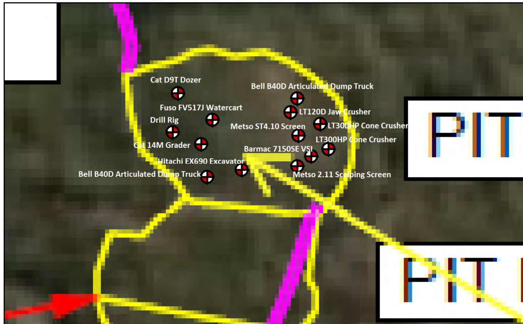
Figure 9: Assumed source locations of scenario 5 – Quarry crushing process with ROM in the south pit.
